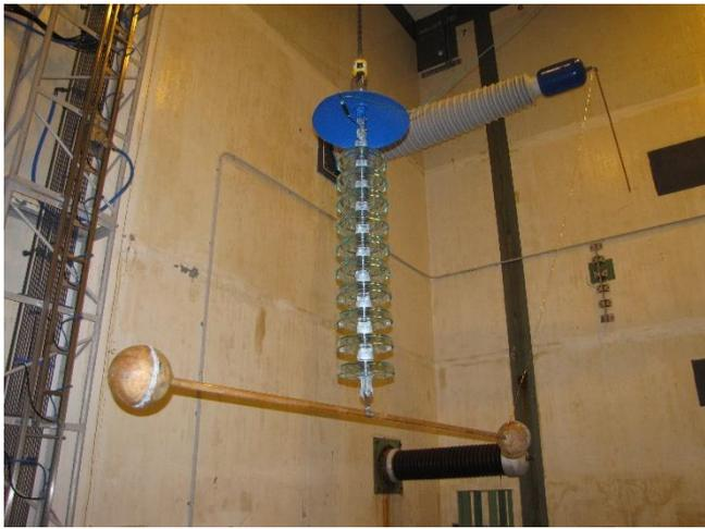
Fig. 2. Glass insulator string in test position.
